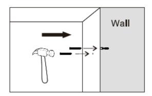
After fitting the wall plugs, insert the screw and tighten, DO NOT tighten the screw fully to the wall surface.
